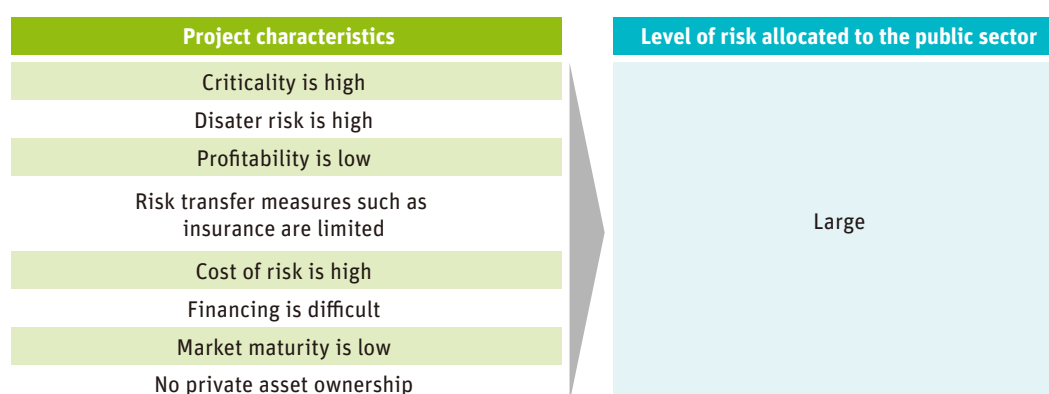
Figure 6.3 Principles of Disaster Risk Allocation to the Public Sector in PPP Projects
