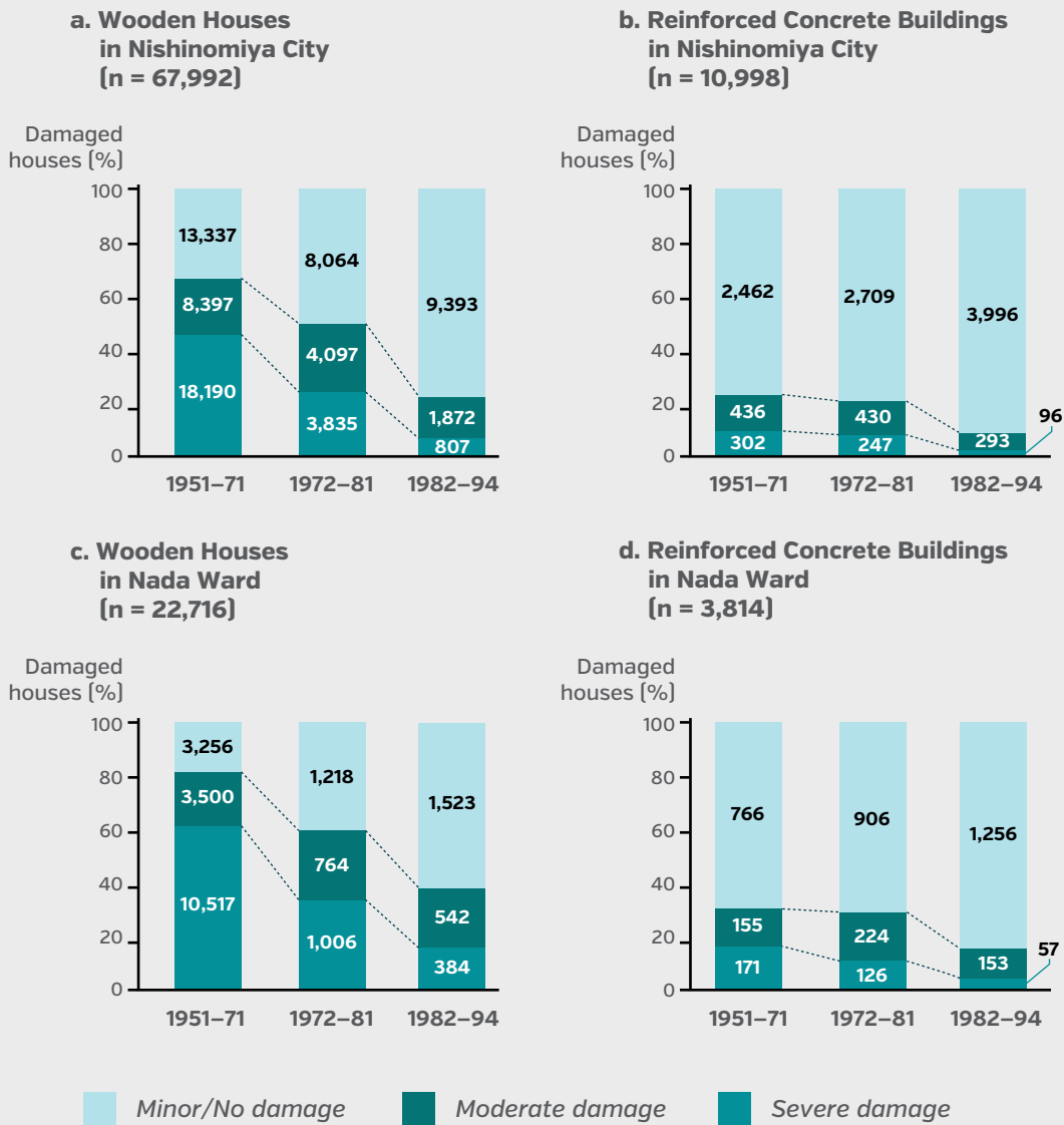
Figure 1.2 Damage to Building Structures in the Great Hanshin-Awaji Earthquake, by Period of Construction
